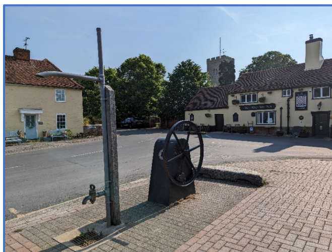
The Goldhanger village well, a rare example of an artesian well with a wheel pump, drilled in 1921 to a depth of 60 metres into the water-bearing chalk deep below the village.
